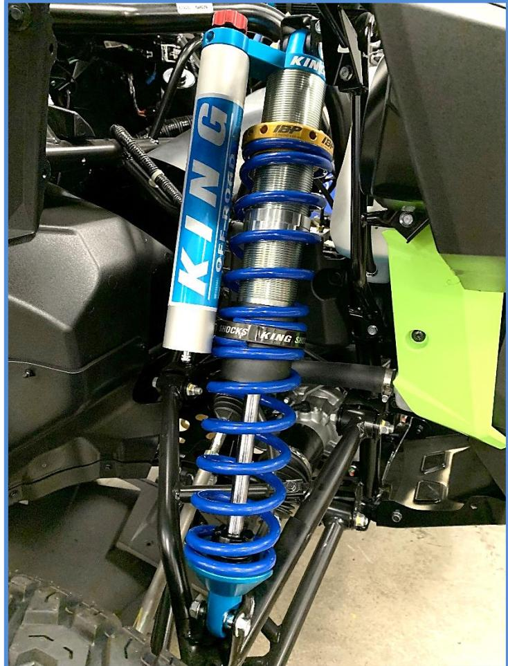
**Double check your install, make sure the shocks are mounted properly and all hardware is tight. Recheck the hardware after 50 miles and periodically after that as part of routine maintenance.**
