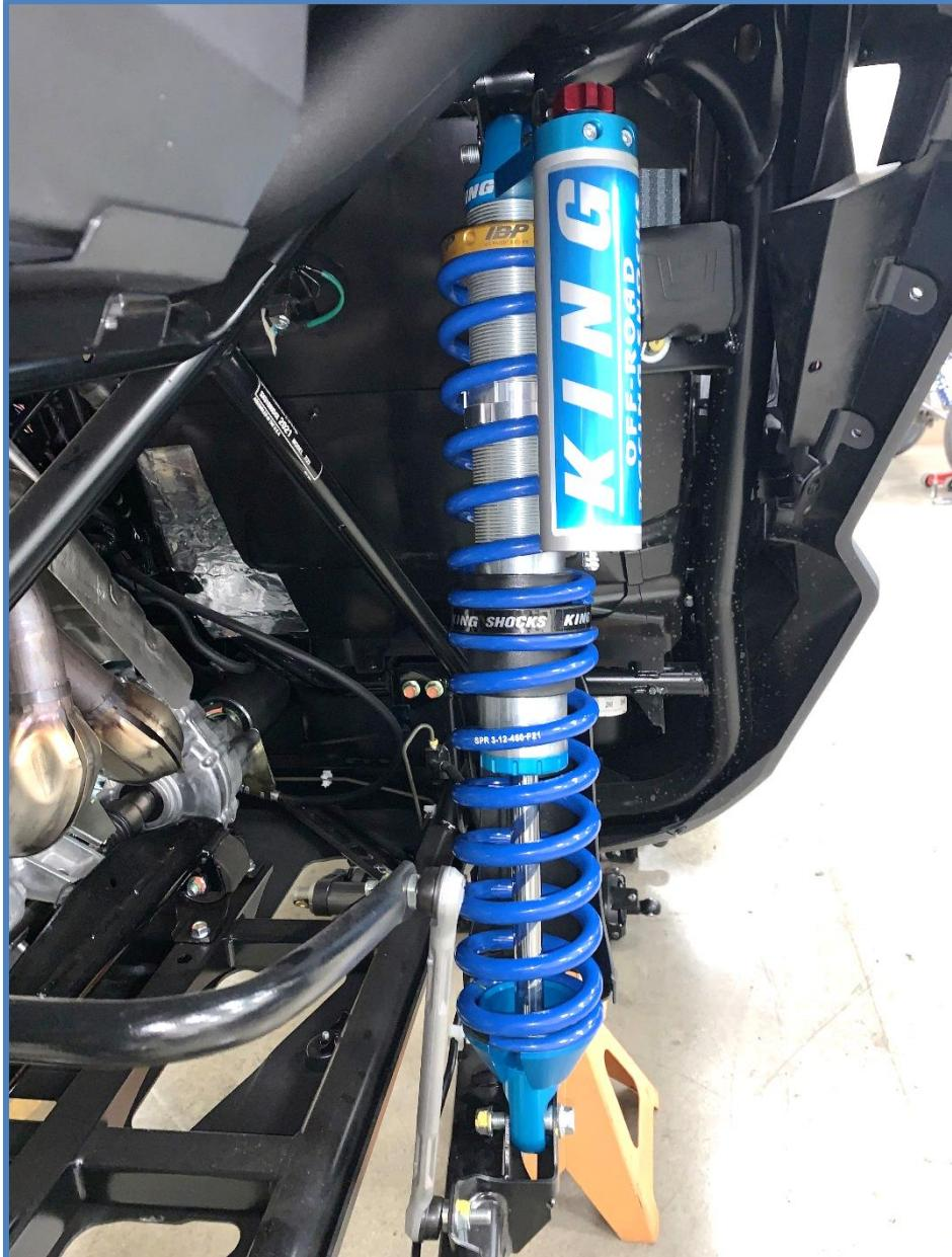
**Double check your install, make sure the shocks are mounted properly and all hardware is tight. Recheck the hardware after 50 miles and periodically after that as part of routine maintenance.**
