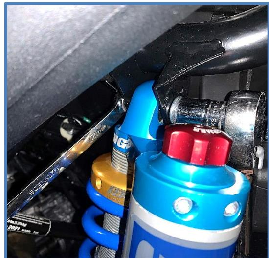
3. Place the rod end in the lower mount with the shaft guard facing forward, install the factory hardware and tighten to factory specs.
