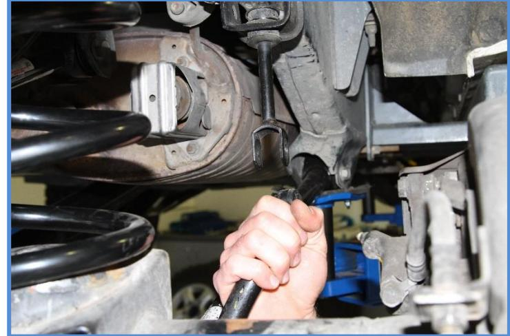
3. Install King Shocks - Remove the nut, washer, blue retaining washer and upper bushing. Insert the pin into the upper mount making sure the taller bushing is on the bottom next to the cylinder.
