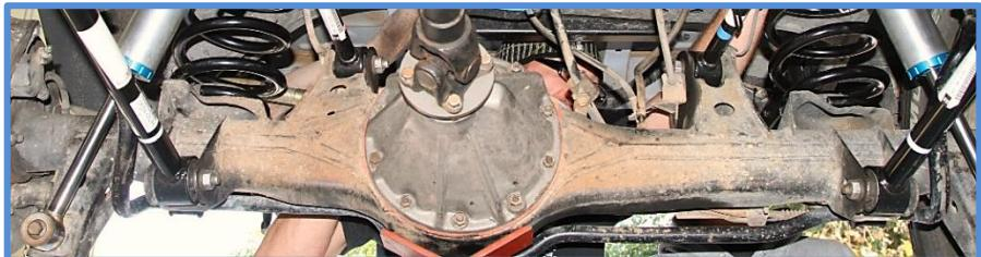
**Remote reservoir applications require welding the reservoir mounts. Do Not Weld on vehicle with shocks installed. All welding must be performed by a certified welder. Reservoir location is up to the customer, be sure to check any clearance issues with hoses/reservoirs and moving suspension components before final install.**
