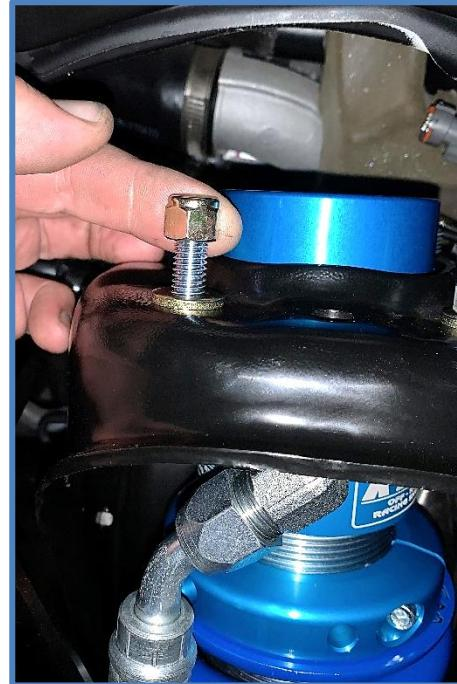
11. Maneuver the rod end onto the lower mounting stud while prying down on the sway bar. Once the rod end is installed, make sure bearing spacers and bushings are properly positioned and install the factory bolt. Tighten the lower bolt to factory specs.
