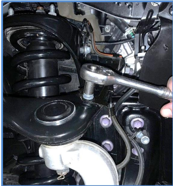
2. Unbolt the ABS/brake line bracket on the frame and spindle using a 12mm wrench or socket.
