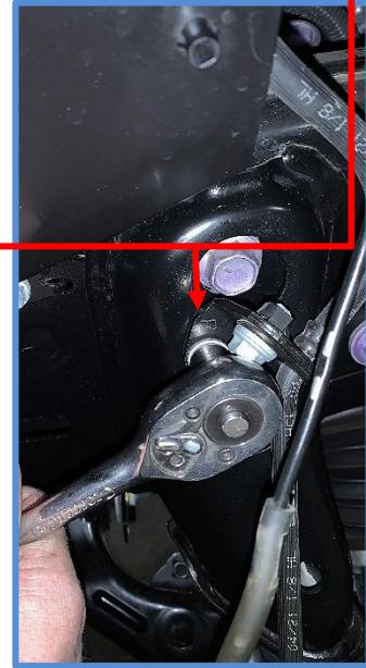
3. Disconnect wire going to the top of the shock. Start by releasing the clips on the connector housing.
