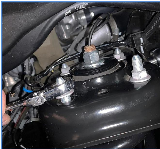
8. Remove the lower mounting bolt using a 22mm socket.
