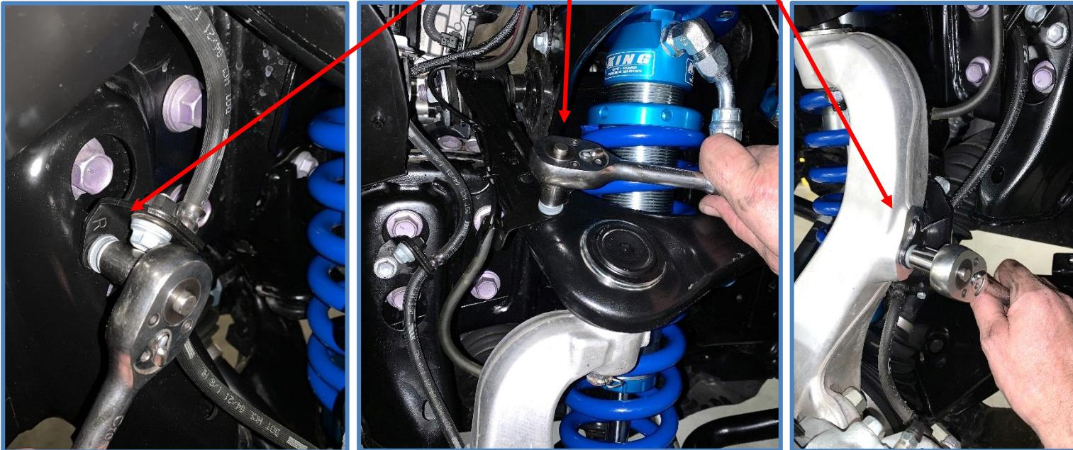
15. **Mount Reservoirs** – First attach reservoir clamps to the reservoir brackets using the supplied 1/4 x 1/2" BHCS (CB2420). Apply red locktite to the threads and attach clamps to brackets as shown below.
