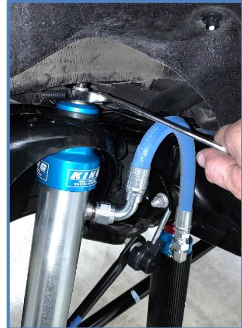
**Important Note:** The rubber bushings on your King shocks have raised center sections that should be facing each other when installed on vehicle. Taller bushing should be on bottom next to cylinder. The silver washer between the rubber bushings represents the material thickness of the upper shock mount. It's important to tighten the nut only until the rubber bushings start to compress. There should be approximately 1/8 – 3/16" of the mounting pin protruding above the nut.
