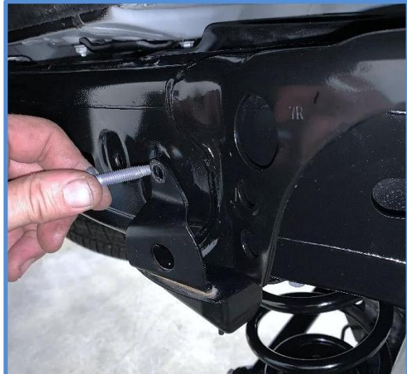
11. Slide the reservoir bracket over the reservoir, then place the bracket over the backing plate as shown below. Install the two short 8mm bolts (CB3825) into the backing plate and install the longer 8mm bolt (CB3824) through the bracket and thread into the existing bump stop hole in frame where you just removed the factory bolt. Tighten all bolts using a 12mm wrench or socket.
