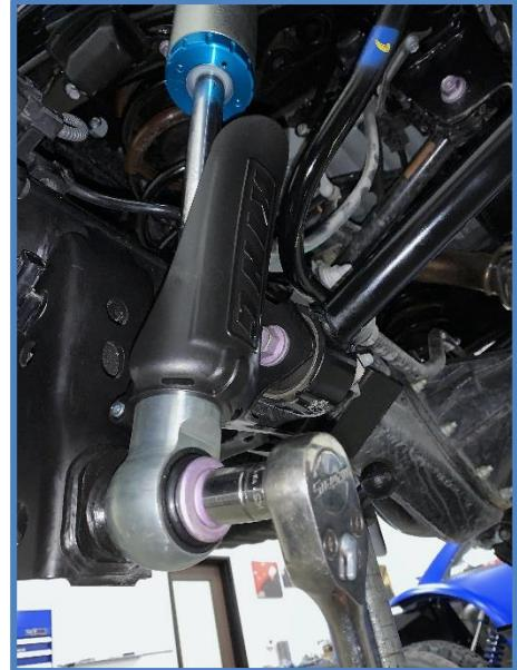
**IBP SHOCKS with WELDED ROD ENDS – USE PROVIDED HARDWARE!**
